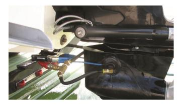
9. To kill mussels in the engine cooling system, use appropriate attachment (e.g. fake-a-lake) connected to the pressure wash unit or other hot water source. Start the engine and make sure adequate water flow is provided to engine cooling system. Run ambient temperature water to allow the engine to warm up, and watch temperature gauge to ensure proper cooling is taking place. Engine manufacturers have preliminary recommendations that inlet
